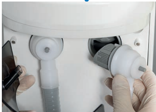
SURGICAL SUCTION FILTERS FOR EACH HOSE
