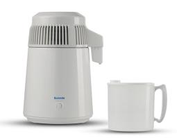
Water distiller for obtaining distilled water by boiling and subsequent steam condensation. It distils 0.7 L of water per hour. 4-litre capacity. It fulfils the safety and electromagnetic compatibility (2014/30/EU) and low voltage (2014/35/EU) tests.
